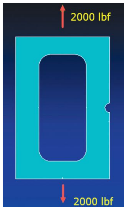
Figure 1: Original damage dressed to a notch shape.
