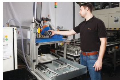
The "Knight concept" allows KUKA's robots to be implemented or removed as needed. Image courtesy of KUKA.
