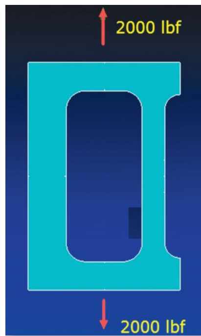
Figure 3: Repair scheme: flared right hand leg to eliminate the notch.
